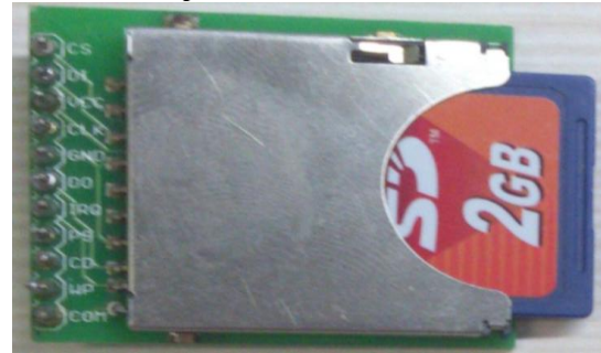
Fig 3: Pins of the SD Card Breakout
