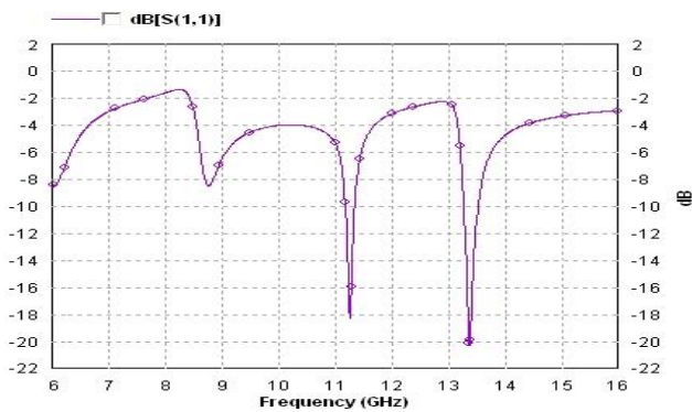
Fig 3: Reflection coefficient of RMPA
