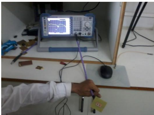
(b) S_{11} measurement setup
