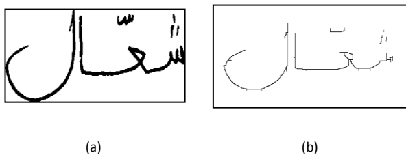
Fig 4. Producing spurious tails (a) Arabic handwriting word 'shaal' (شعال) before thinning; (b) the word 'shaal' (شعال) is being thinned using the Zhang and Suen parallel thinning algorithm.
