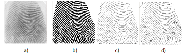
Fig. 15: Result of bifurcation type minutiae extraction applied to an image with median filter pre-processing. a) original image; b) binarized image; c) sharpened image; d) extraction of minutiae.
