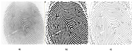
Fig. 13: Result of Stentiford thinning. a) fingerprint; b) binarization; c) thinning.
