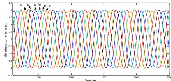
Fig 2: Six phase current waveforms during no fault condition
