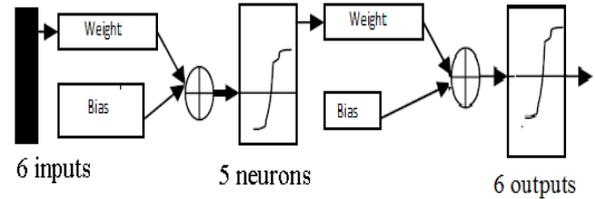
**Fig 4: Structure of ANN based fault distance locator**
