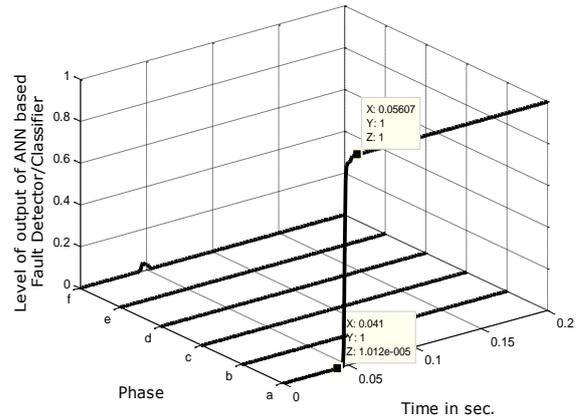
Fig.7: Test result of ANN based FD/C for one conductor open fault ‘a’ at 64 km with  $\Phi_i=180^\circ$  ( $t_i=0.041$ sec.)
