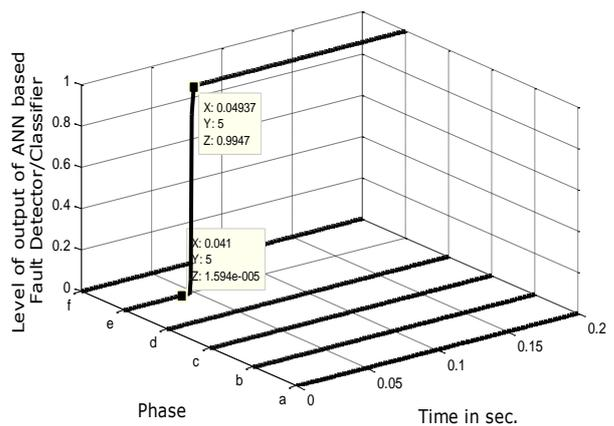
Fig.8: Test result of ANN based FD/C for one conductor open fault ‘e’ at 45 km with  $\Phi_i=180^\circ$  ( $t_i=0.041$ sec.)
