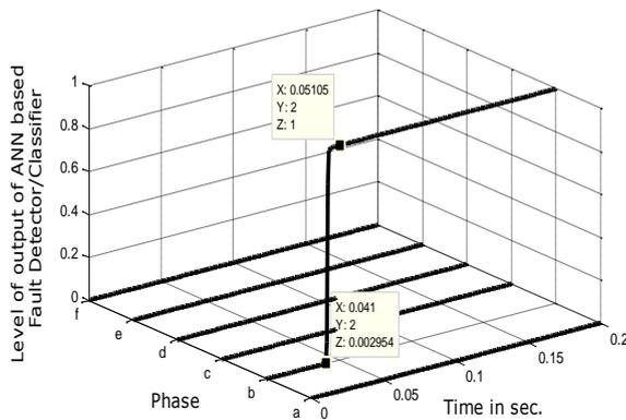
Fig.6: Test result of ANN based FD/C for one conductor open fault ‘b’ at 2 km with  $\Phi_i=180^\circ$  ( $t_i=0.041$ sec.)
