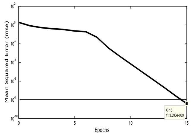
**Fig 5: Training of ANN based fault detector and classifier for one open conductor fault**
