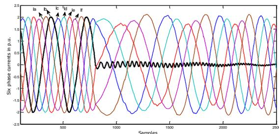
Fig 3: Six phase current waveforms during one conductor fault on phase “b” at 45 km with  $\Phi_i=0^\circ$
