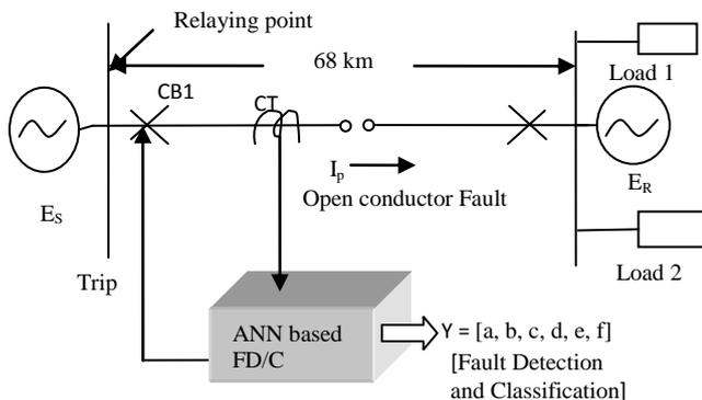
Fig 1: Single Line Diagram Of Six Phase Transmission Line under study
