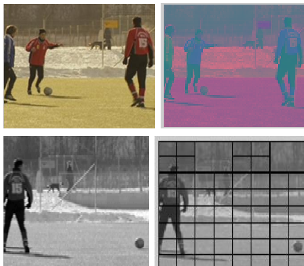
Fig.8 Process of Encoding - Soccer video (Colored Reference frame, current frame , YCbCr frame, gray frame and quad-tree decomposition)
