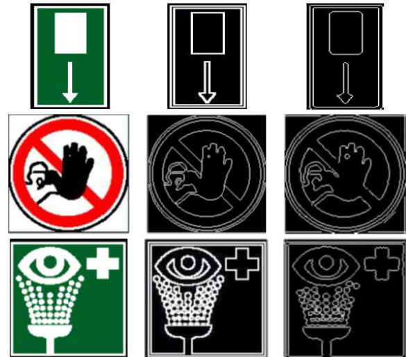
Fig 4: from left to right: the initial image, the image segmented manually and the results of segmentation using the combination of operators founded by the agent OA
