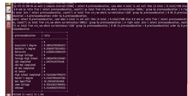
Figure 8: Snapshot of complex query (using joins, group by) on Hadoop Cluster.
