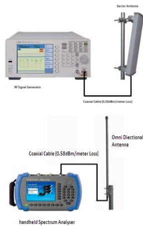
Fig. 1 : Transmitter and Receiver Configuration
