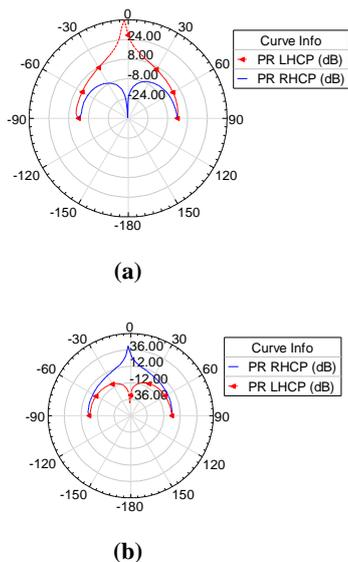
**Fig 5: Polarization ratio radiation pattern for E plane at 5.788GHz (a) LHCP mode (b) RHCP mode.**
