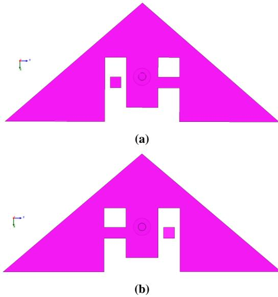
**Fig 2: Geometry of simulated prototype antenna: (a) LHCP mode. (b) RHCP mode.**
