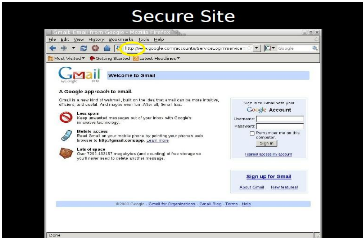
Fig 3 Result of the sslstrip attack.
