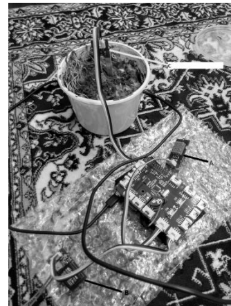
Fig 2: Connection setup in hardware side
