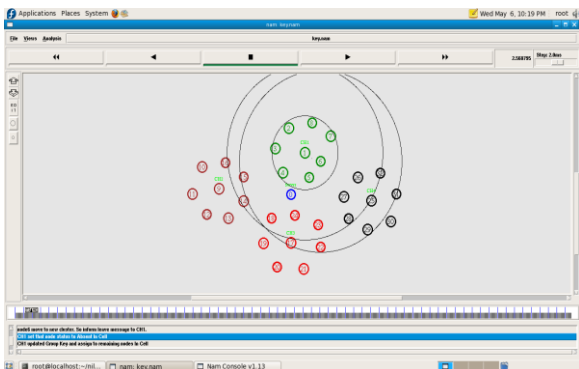
Fig 5: Node 6 sending leave request to Cluster head1 (CH1)
