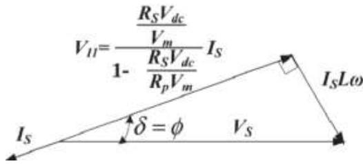
Fig.5. Phasor diagram depicting the steady-state component of the proposed voltage-sensorless system.
