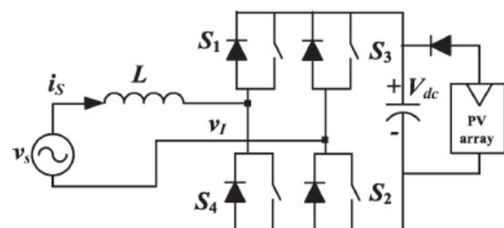
Fig.2 1 phase single stage grid connected PV system
