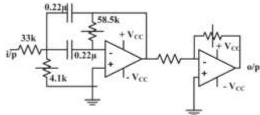
Fig. 4-Circuit diagram of analog implementation of BPF
