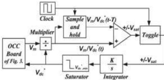
Fig. 6. block diagram of MPPT realization
