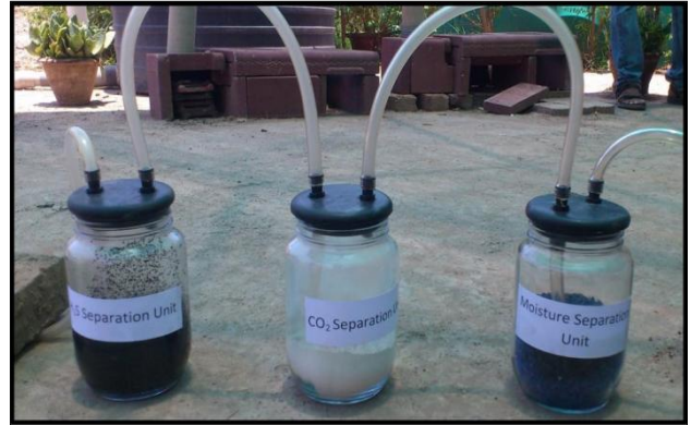
Fig 2. Biogas scrubbing unit
