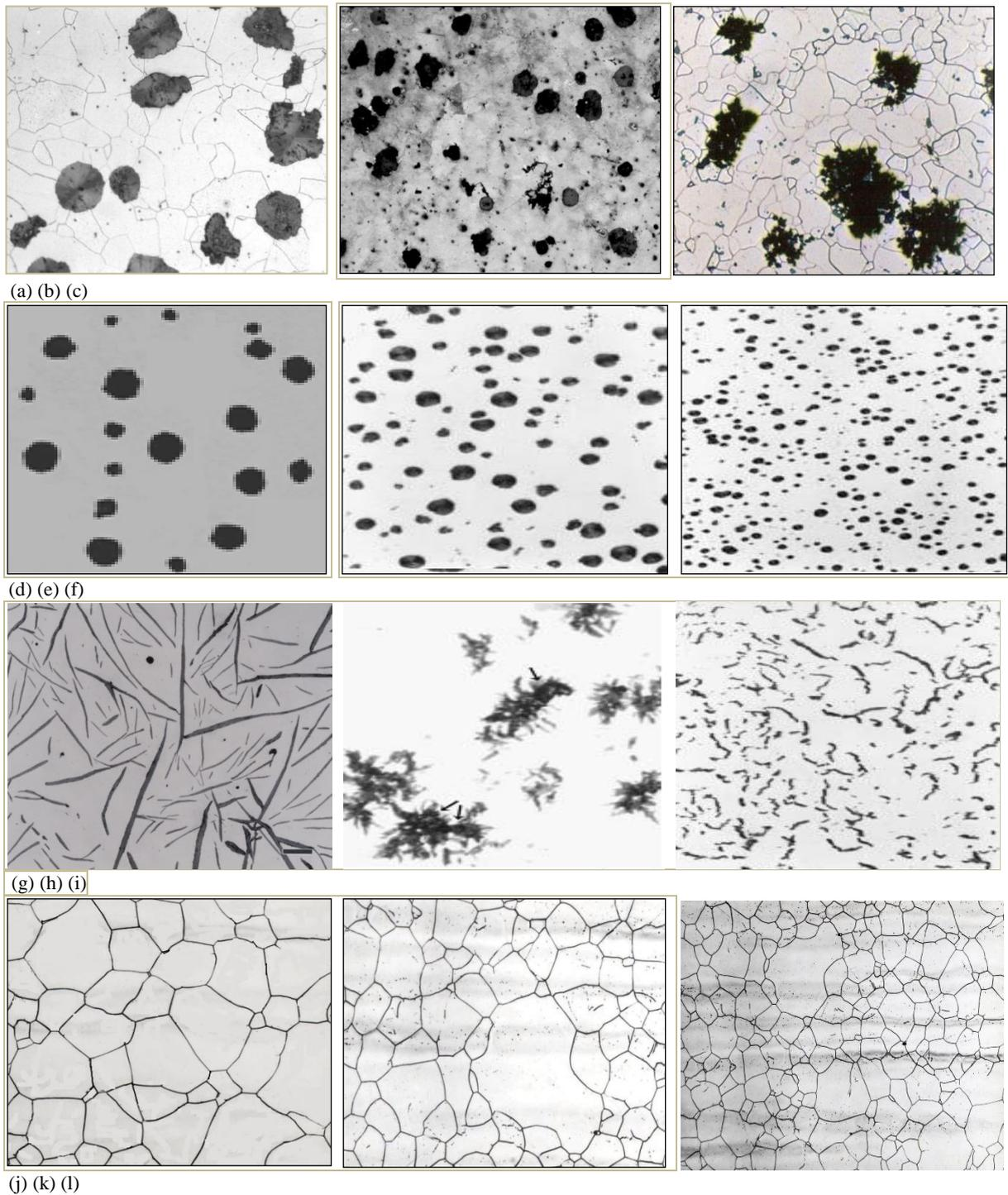
**Fig.4: Sample microstructure images of cast iron: (a)–(i) Two-component and (j)–(l) One-component material microstructure images. Wt. percentage of C in microstructure 4(a)-5%, 4(b)-2.9%, 4(c)-4.2%,4(d)-2.9%,4(e)-3.5%.**
