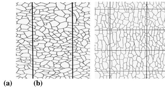
**Fig.1: Counting procedures for determining global stereological parameters in single-component microstructures: a) isotropic grain structure, counting of number of intersection points of boundary with test line,  $P_L$ ; b) oriented grain structure, counting of intersection points with test lines oriented in and perpendicular to orientation directions,  $P_{L(or)}$  and  $P_{L(perp)}$  [14].**
