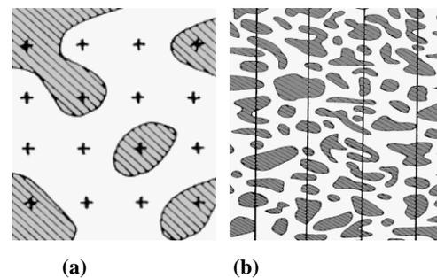
**Fig.2: Counting procedures for determining global stereological parameters in two- and multi-component microstructures: a) counting hit points with a point grid in two fields for determining the volume fraction; b) counting the number of intersection points of test lines with  $\alpha\beta$ -interface,  $P_{L(\alpha\beta)}$  [14].**
