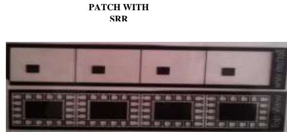
Fig 6: HFSS Design taken printed on Glass Sheet
