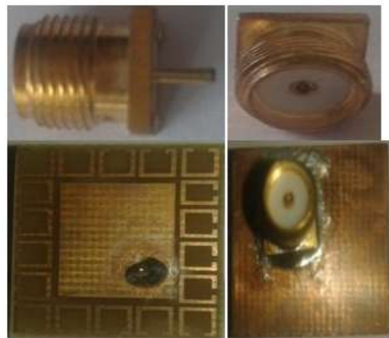
Fig 8: SMA connector and Soldering of SMA connector on antenna
