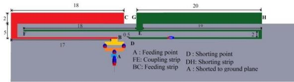
Figure 1(b): Detailed dimension and structure of the proposed antenna. (Unit mm)
