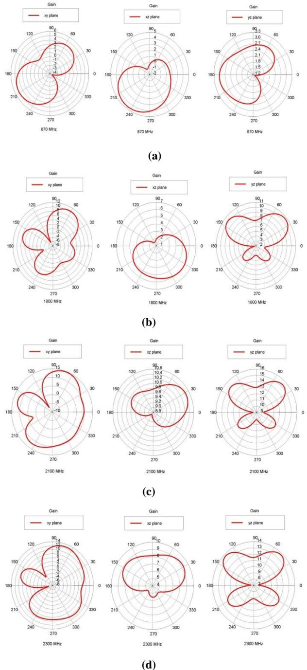
Figure 5: Measured 2-D gain patterns at (a) 870 MHz (b) 1800MHz (c) 2100 MHz (d) 2300MHz for the proposed antenna
