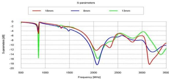
Figure 2: S parameter of the proposed antenna at different coupling lengths.
