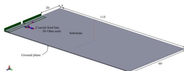
Figure 1(a): Geometry of the low-profile antenna for ten-band operations in the internal smartphone applications
