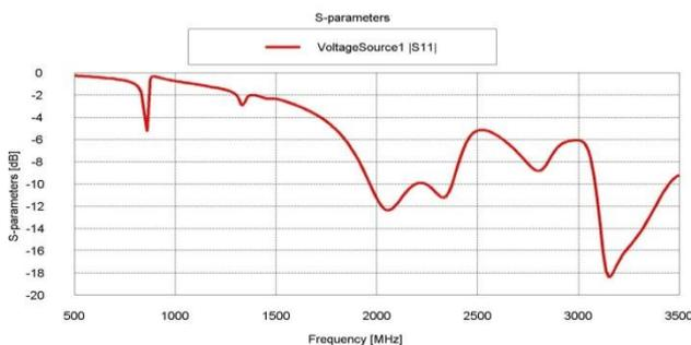
Figure 3: S parameter of the proposed antenna
