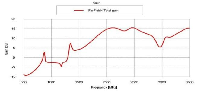
Figure 4: Gain of the proposed antenna
