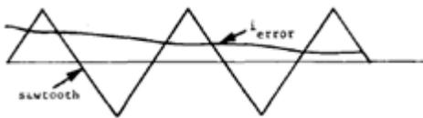
Fig 4 Triangular reference current.
