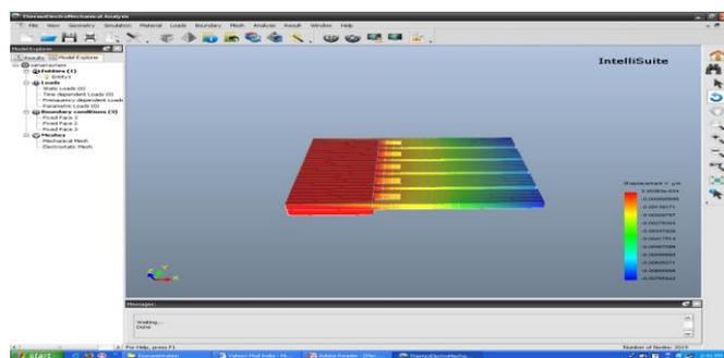
The sensitivity of the device is directly proportional to the length by thickness ratio ( $L/t$ ) of the microcantilever. Therefore, the longer and thinner the microcantilever is, the greater is the sensitivity of the device.
