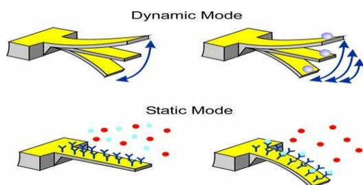
**Figure 2 : Schematic drawings of the two possible modes of operation of cantilever-based sensors.**
