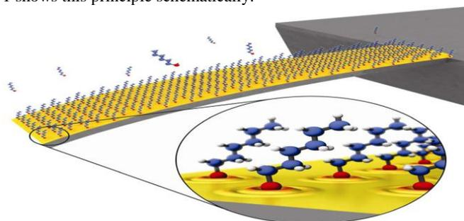
**Figure 1.** As molecules selectively bind to one surface of the cantilever, the structure is deflected due to the generated surface stress.
