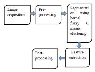
The system consists of the following blocks. The raw data is passed through the system as numerical data or in the form of waves. Applicable techniques are applied to get the preprocessed data. Further, the data is passed through the clustering phase, which returns the cluster centers. Feature extraction is then performed to obtain the attributes that can downright exemplify a given instance. Next a post processing is used to enhance the quality of the final segmented image
