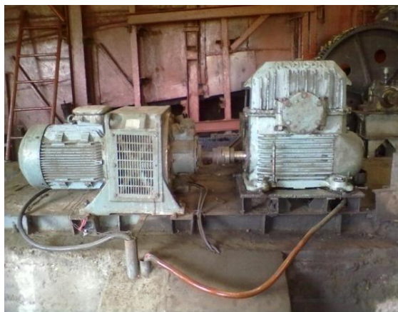
Fig.2 Photograph of implemented eddy current drive in M.S.S.K Sugar Industry
