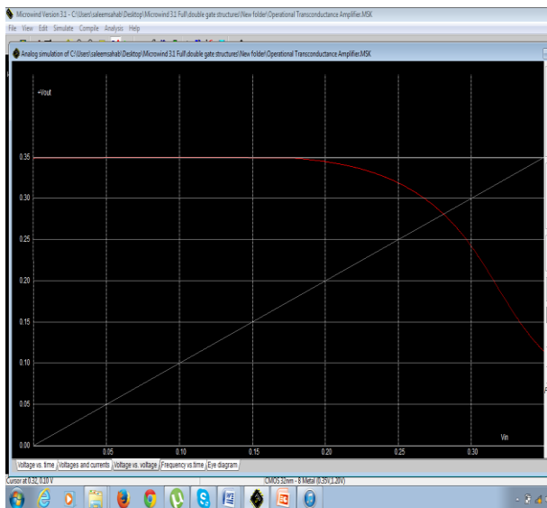
Fig.3.3 (a) Output DC response of OTA DG-MOSFET
