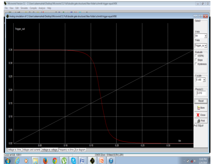
Fig.3.2 (b) Output DC response of Schmitt triggers using DG-MOSFET
