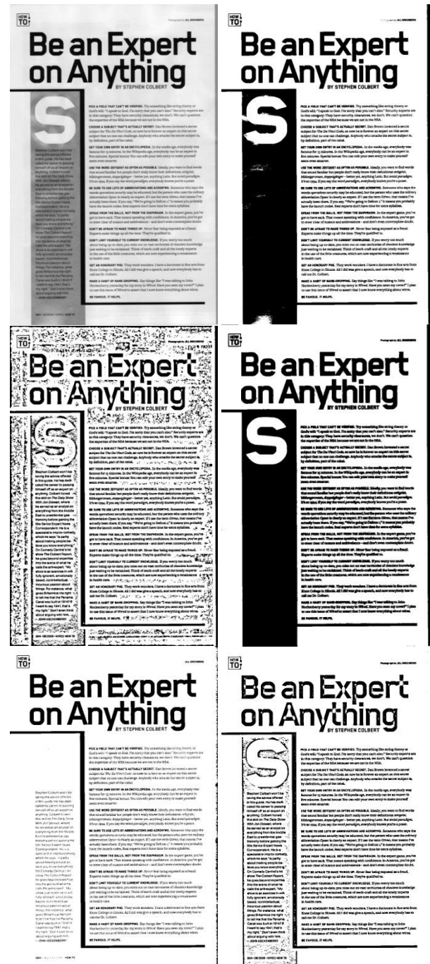
Figure 3- (Clockwise from top) - Input grayscale image, Otsu's output, Wolf's output, Output of the proposed method, Sauvola's output, Niblack's output.
