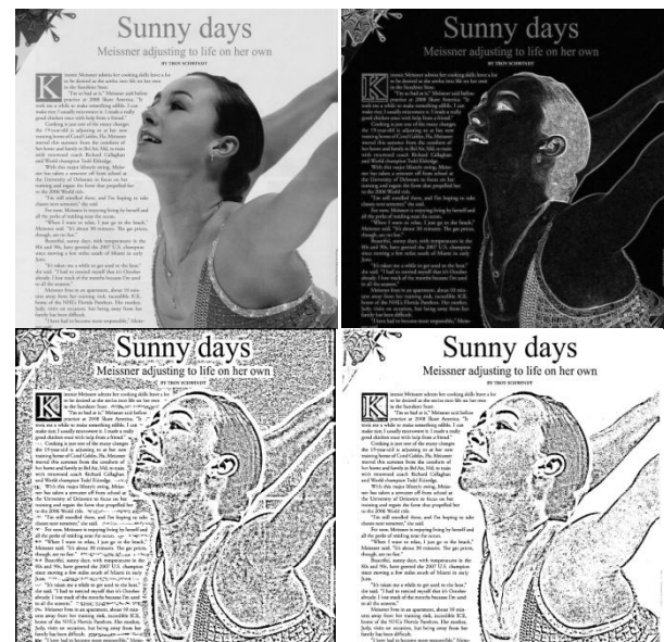
Figure 1- (Clockwise from top) - Input grayscale image, Contrast map of the input image, Output of the proposed method, Output of Niblack's method.
