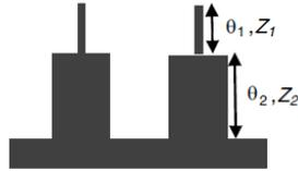
Fig. 8. Proposed inverted stepped-impedance BPF
