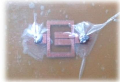
Fig.10 (b). Photograph of the fabricated resonator on an FR-4 substrate.
