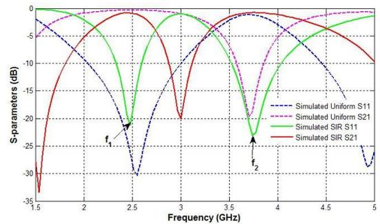
**Fig. 7. The resonant frequencies of the uniform and the stepped resonators.**
