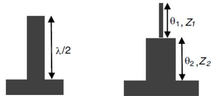
**Fig. 6. The uniform (left) and the inverted stepped (right) resonators**
