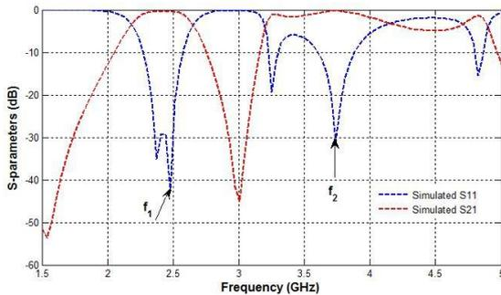
Fig. 9. Simulation results of the dual-band inverted stepped impedance bandpass filter.
