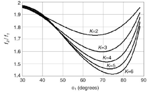
**Fig. 5. Variation of the second resonant frequency with the impedance ratio  $K$ .**
