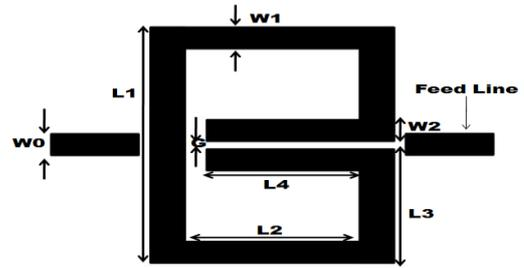
Fig. 10(a). Proposed compact stepped-impedance resonator
