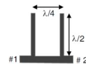
Fig .2. Conventional half-wavelength open-circuited stub BPF structure.
