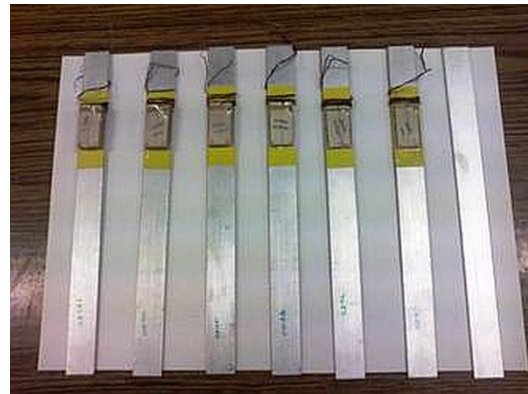
Fig. 9: The actual specimens with variation of thickness of PZT
