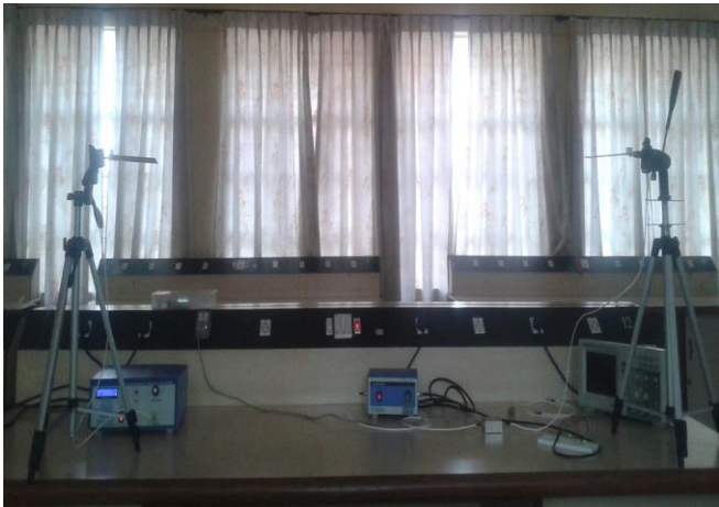
Fig.3. Experimental setup that depicts WPT using Yagi-Uda Antenna on both Transmitter and Receiver end.
