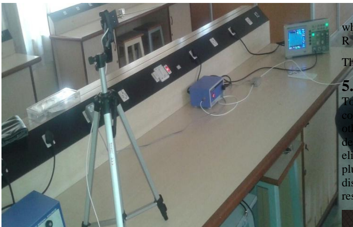
Fig.4. Experimental setup that depicts WPT using Yagi-Uda Antenna on Transmitter end and Monopole Antenna on Receiver end
