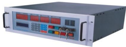
Fig 5: Hardware Based CDT Generator
