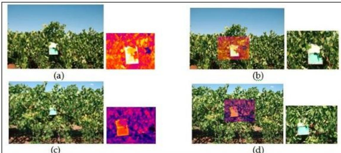
Figure 2: Outcomes of SIFT based registration algorithm (no matching key- points)
