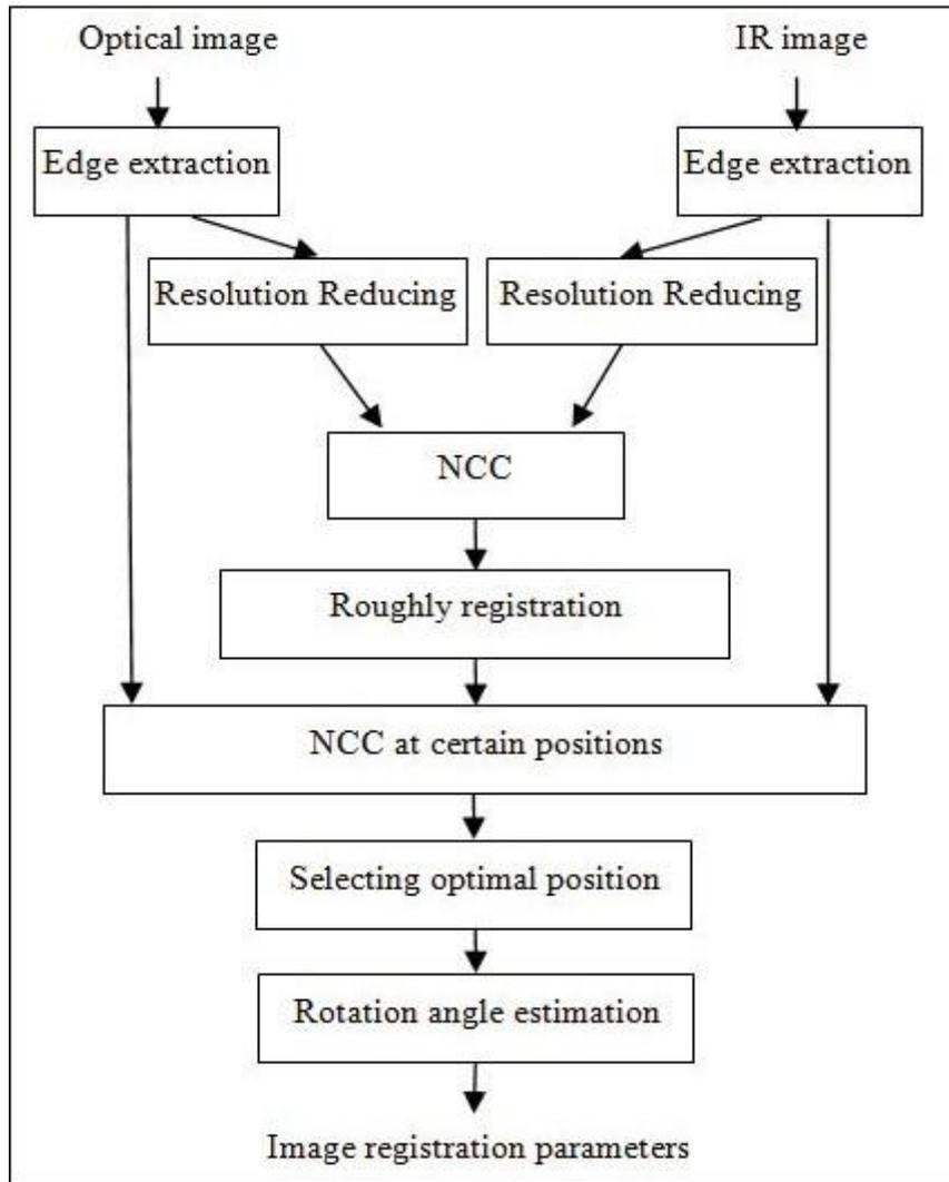
Figure 3: Flow Diagram of variable resolution algorithm based on NCC
