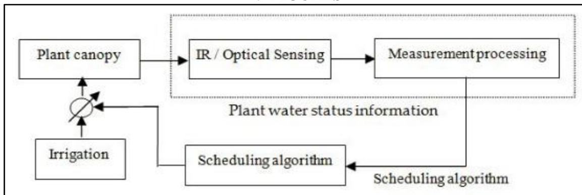
**Figure 1: Illustration of irrigation actuation via a plant based sensor**
