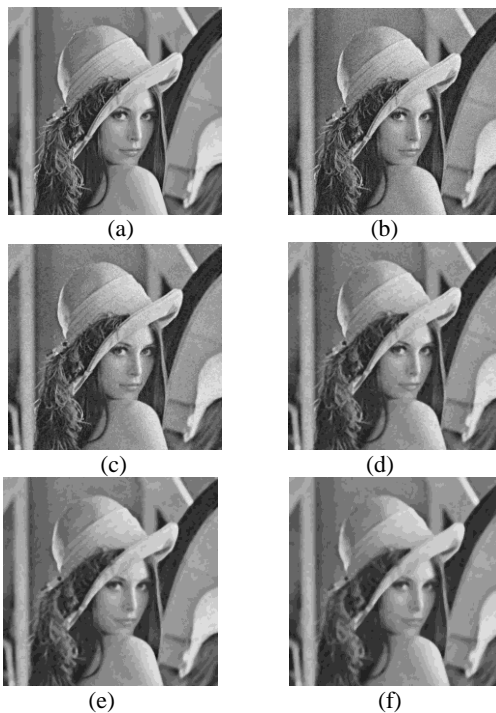
Figure 1. Restoration results (a) Noise-free image 'Lena' (b) Image corrupted image with Gaussian noise with \sigma = 15 (c) Result using 3 \times 3 AWMDF (d) 5 \times 5 AWMDF (e) 7 \times 7 AWMDF (f) 9 \times 9 AWMDF
