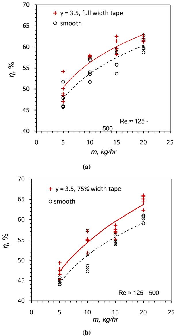
**Fig. 3. Thermal efficiency versus the flow rate (a) Full width twisted tape, (b) 75% width twisted tape.**
