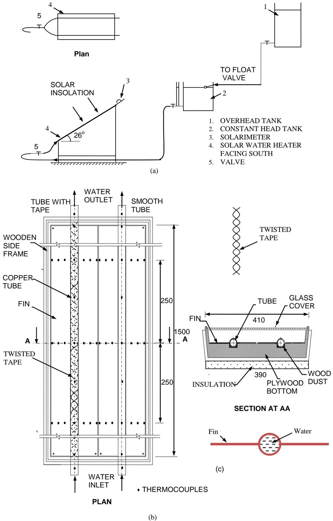
Fig. 2. (a) Schematic of experimental setup, (b) solar water heater, (c) copper tube with brazed fins.
