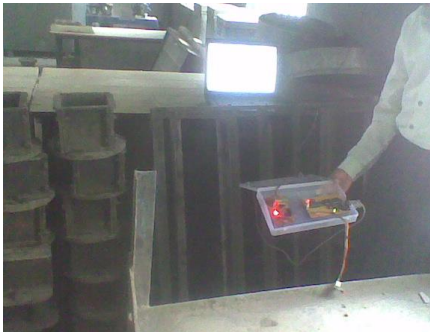
Figure 2 Experimental Set Up For Vibration Measurement of Vibrator Table Tested In Civil Engg Lab
