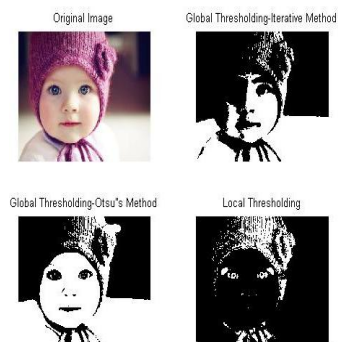
Fig 4: Resultant threshold value and corresponding threshold segmented RGB image.
