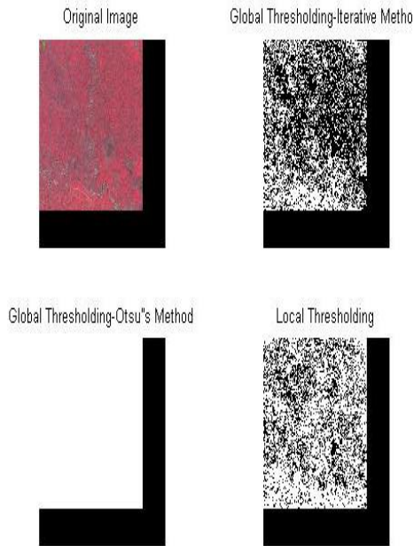
Fig 2: Threshold segmentation on multispectral image of Bareilly region.
