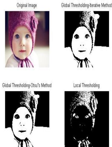
Fig 4: Resultant threshold value and corresponding threshold segmented RGB image.
