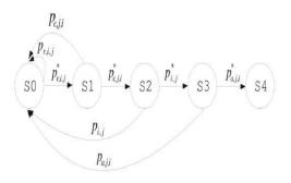
Fig.1 State diagram for the four frame exchange scheme.
