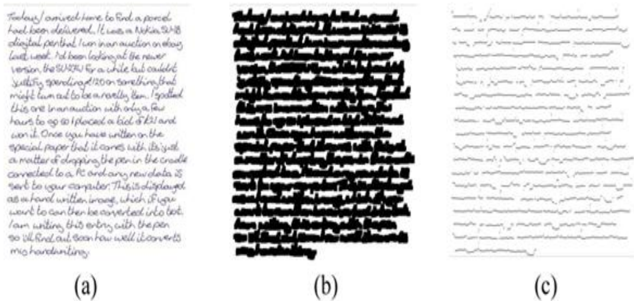
Figure 5.1: Illustration of Partial text-line boundary detection. (a) A handwritten document. (b) Blocked text-lines. (c) Partial boundary lines
