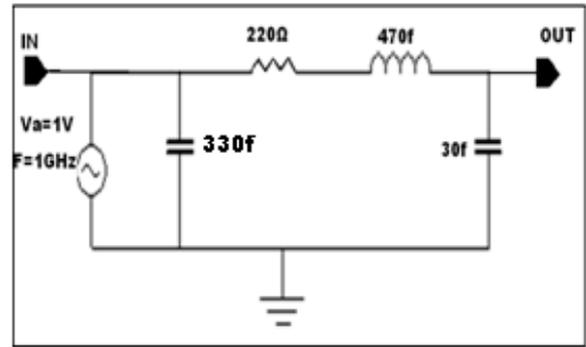
**Fig. 4: Schematic of  $\pi$ -RLC Interconnect Model**
