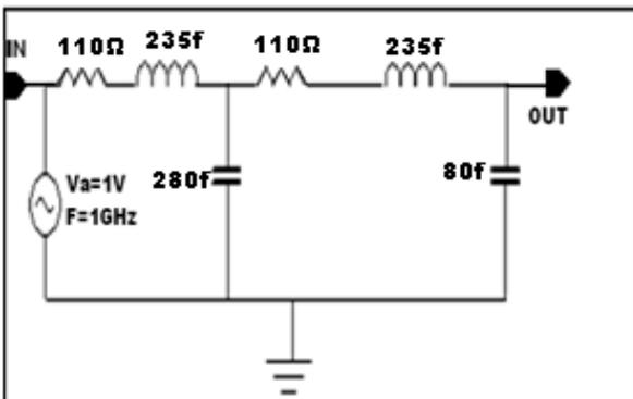
**Fig. 3: Schematic of T- RLC Interconnect Model**
