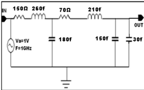
**Fig. 2: Schematic of Reduced RLC Interconnect Model**
