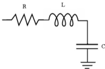
Fig 1: RLC Equivalent Interconnect Model
