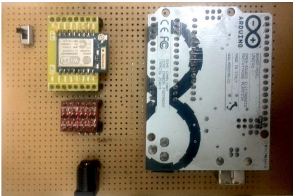
Figure 3: PCB with Arduino® Uno connected to ESP8266 via Sparkfun Level Shifter
