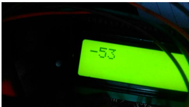
Figure 6: RSSI value alone on LCD
