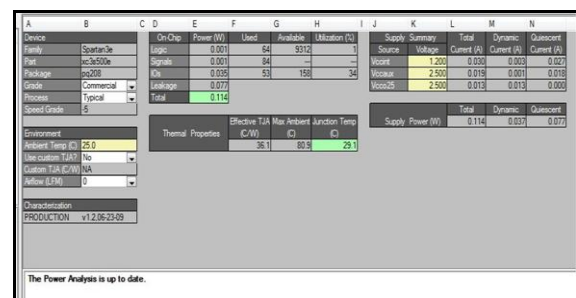
Figure 13: Power dissipation for 16 bit reversible ALU
