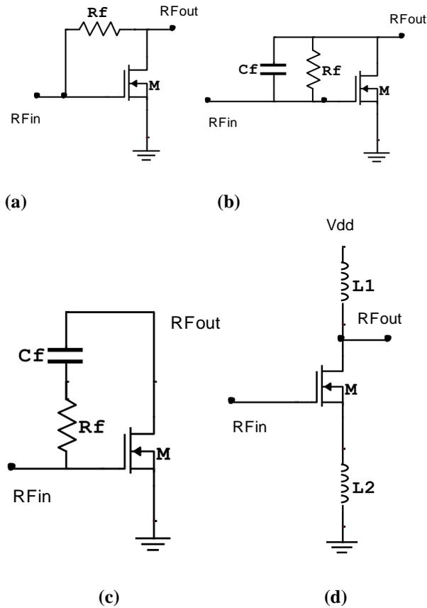
Fig. 2 Feedback topologies a) resistive b) series RC c) parallel RC and d) transformer.
