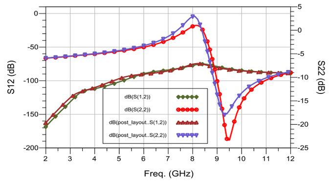
Fig. 8 Input matching simulation
