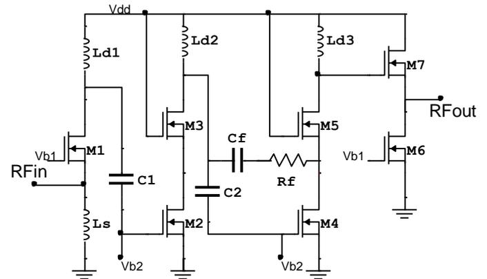
Fig. 3 Schematic of proposed UWB LNA
