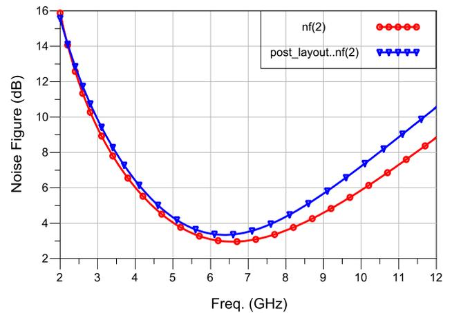
Fig. 9 Noise figure simulation
