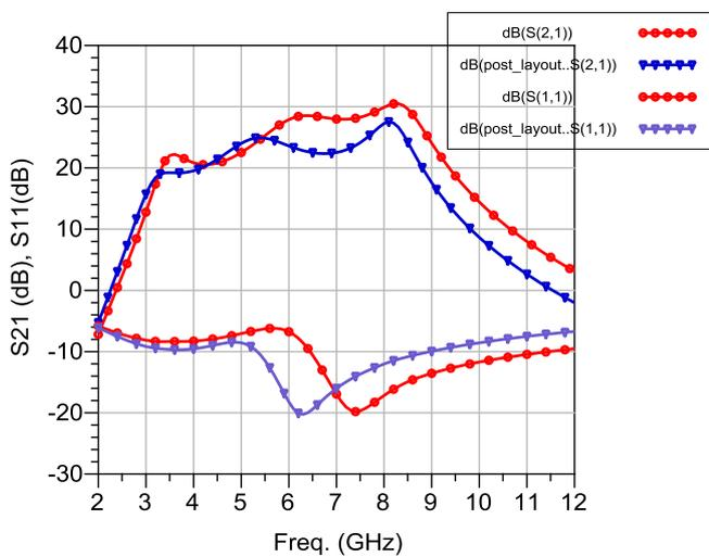
Fig. 7 Power gain simulation
