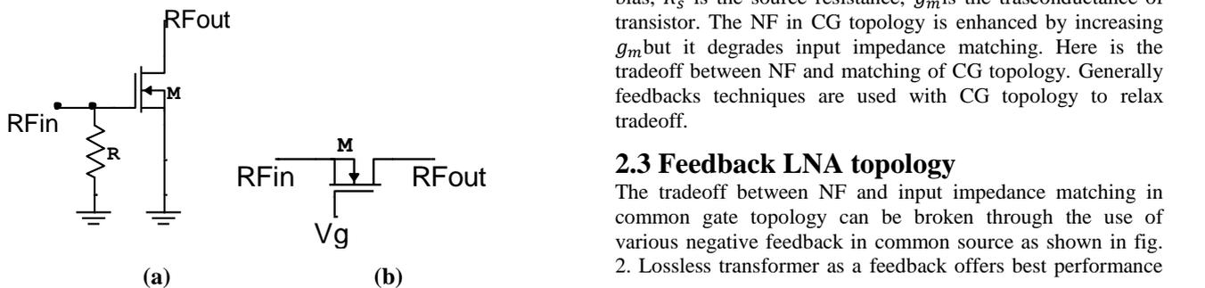
Fig. 1 Wideband LNA topologies a) resistive termination, b) common gate, c) feedback, d) filter and e) distributed
