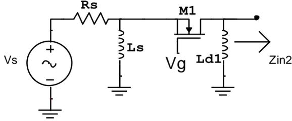
Fig. 4. Common gate first stage
