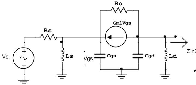
Fig. 5. AC equivalent circuit of CG
