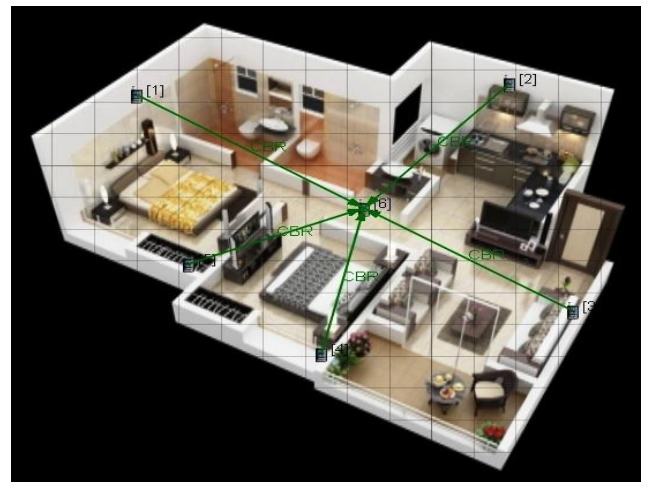
Fig 1: Schematic view of star topology for sensor based housing home using Qualnet Simulator
