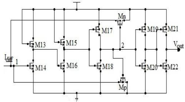
Fig. 3 Schematic of Comparator Stage
