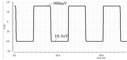
Fig. 7 Output Voltage Swing
