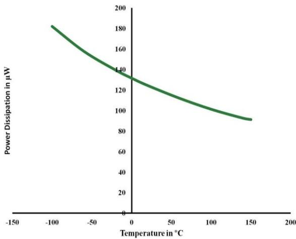
Fig. 11 Variation of Power with Temperature
