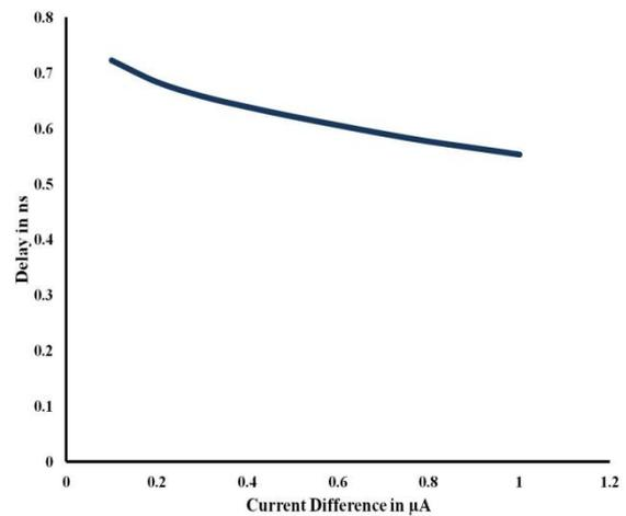
Fig. 8 Variation of Delay with Current Difference
