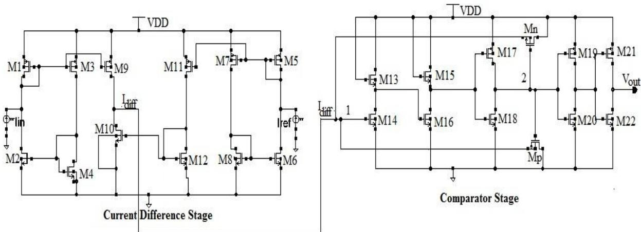
Fig. 4 Schematic of Proposed Current Comparator
