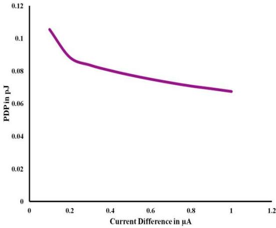
Fig. 10 Plot of PDP against Current Difference
