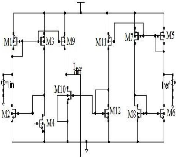
Fig. 1 Schematic of Current Differencing Stage
