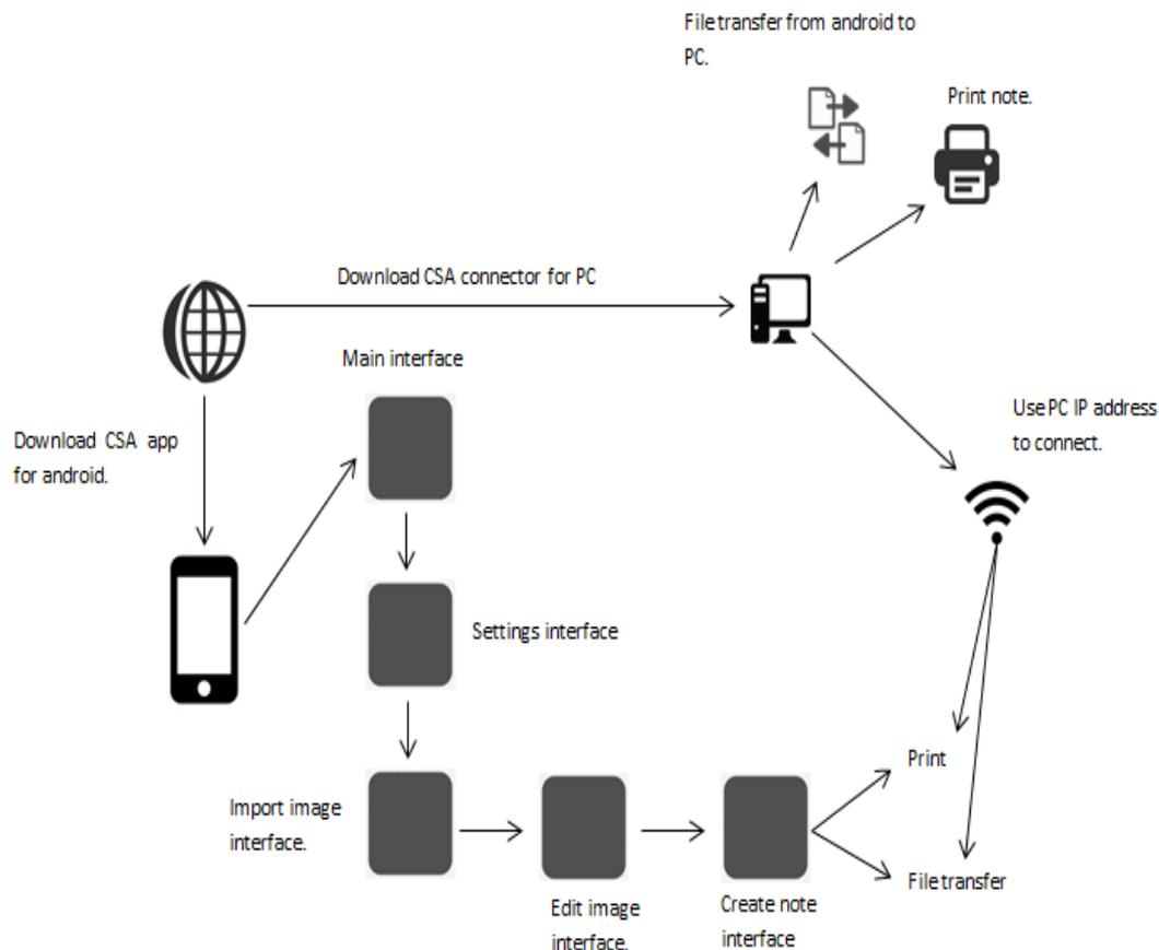
**Fig:1 CSA structure diagram**
