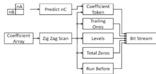
Figure 3. The CAVLC block diagram [2]
