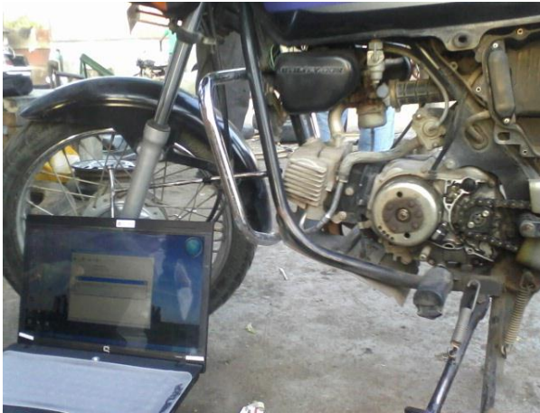
Fig.2: Experimental Setup with audio signal capturing system.
