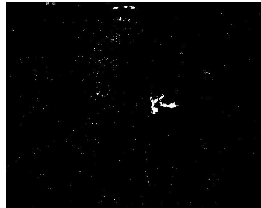
Fig 7: Segmented image indicating the area of smoke intrusion detection
