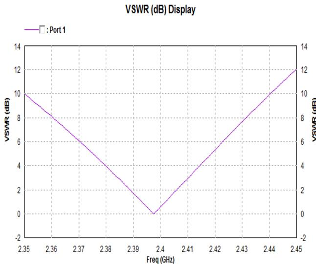
**Fig 8: VSWR (in dB) with the coaxial probe feed Single E-shaped microstrip patch antenna.**
