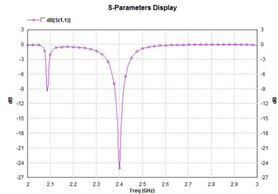
**Fig 5: Return Loss (in dB) of the Microstrip line feed Single E-shaped antenna without optimization.**
