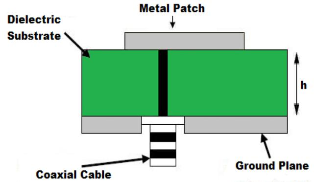
Fig 3: Coaxial cable (Probe) feeding of patch antenna.
