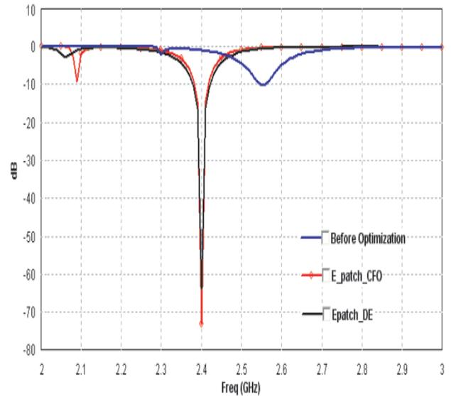
**Fig 6: Return Loss (in dB) with CFO/DE optimization of the Microstrip line feed Single E-shaped patch antenna [10].**
