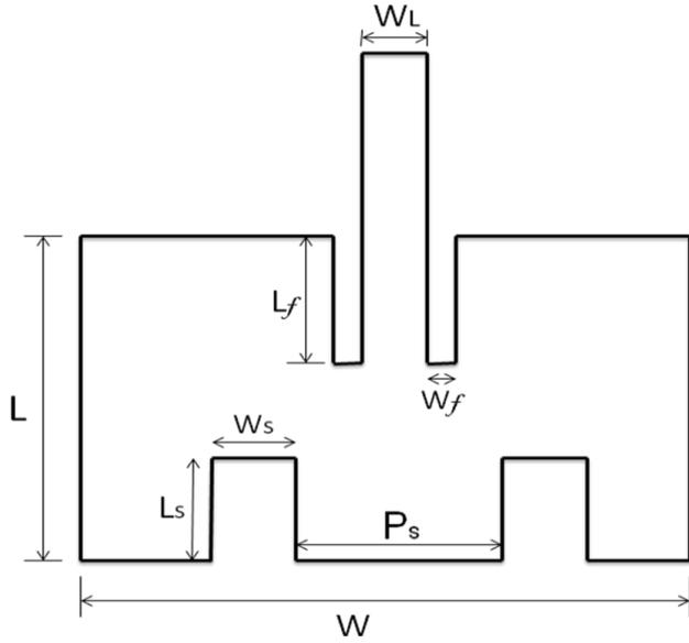
**Fig 4: Geometry of low-profile E-shaped microstrip patch antenna [10]**
