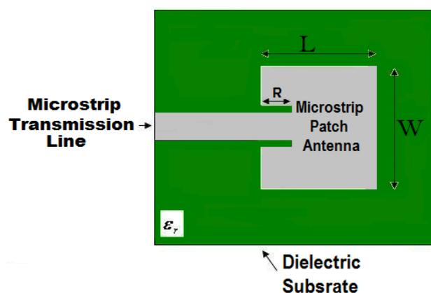
**Fig 1: Rectangular Microstrip patch antenna with an Inset Line feeding.**
