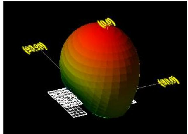
**Fig 10: 3D view of radiation pattern looking along Z axis in the XY Plane.**
