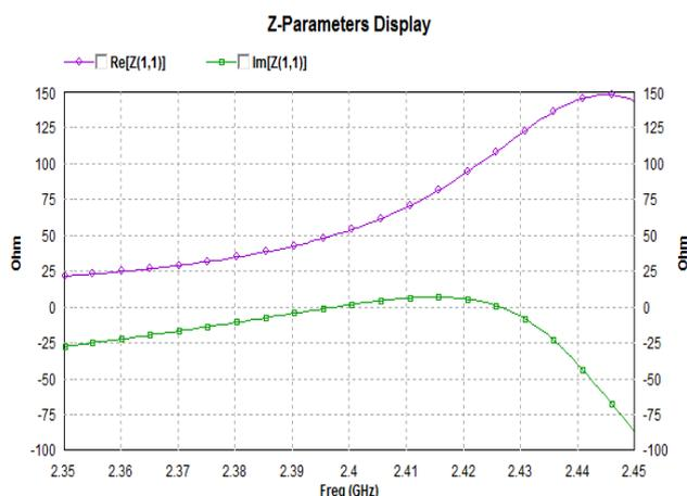
Fig 11: Impedance Plot, which shows  $R=50\Omega$  at 2.397 GHz
