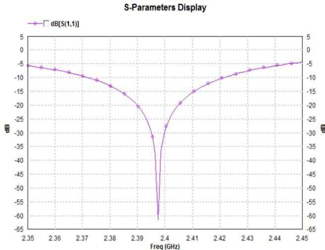
**Fig 7: Return Loss (in dB) of the coaxial probe feed Single E-shaped microstrip antenna.**
