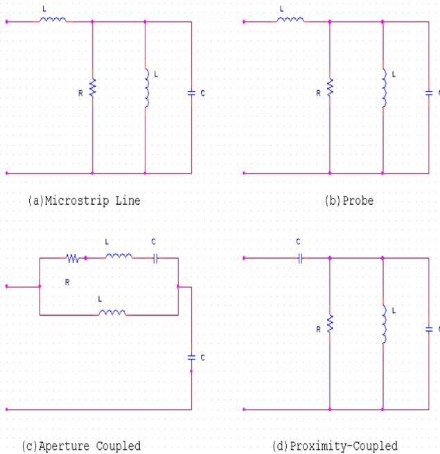
Fig 2: Equivalent circuits of typical feeding methods
