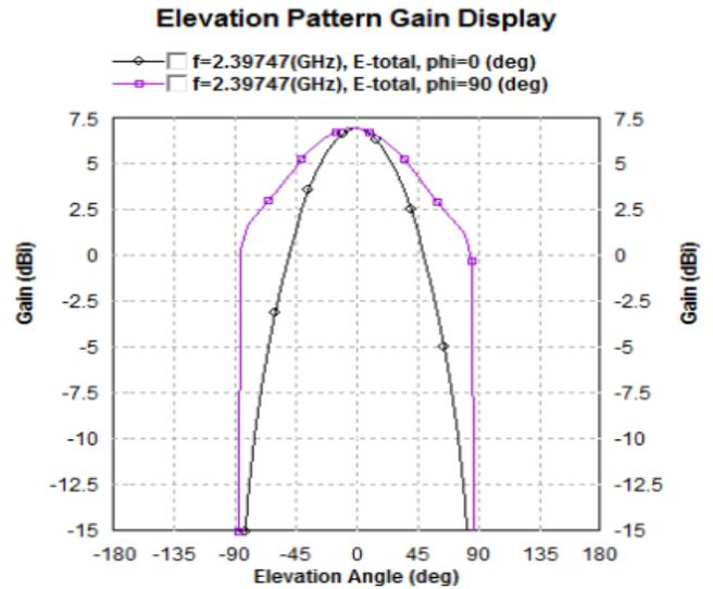
**Fig 9: Elevation pattern for  $\Phi=0$  and  $\Phi=90$  degrees.**
