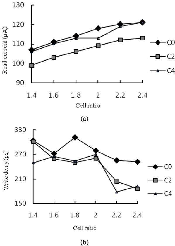
Figure 3: a) Read current and b) Write delay variations with cell ratio for C0, C2, and C4 SRAM cells
