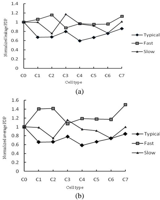
**Figure 8: Normalized power delay product (PDP) variation for (a) leakage power and (b) average power for various SRAM cell configurations**
