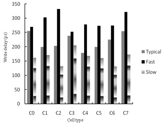
Figure 4: Variation in write delay for different SRAM cells
