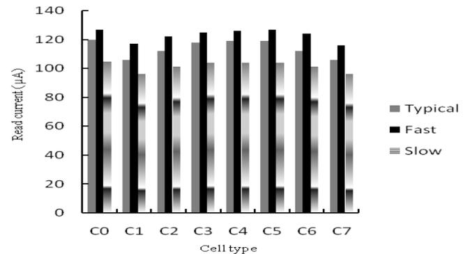
Figure 5: SRAM Cell type versus read current
