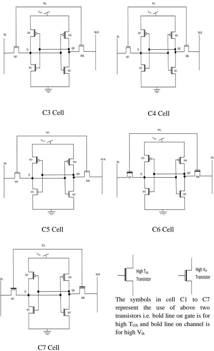
Figure 2: Hybrid SRAM Configurations [12]
