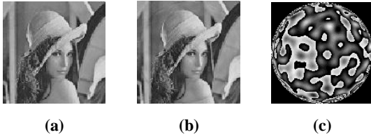
Fig. 1: Example of watermark embedding (a) sample test image Lena (b) the output watermarked image ( p_{max} = 55, \Delta = 1.0, L = 512, PSNR = 51.87 dB) (c) spatial watermark signal
