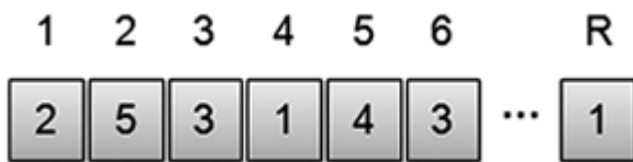
Figure 3 An example chromosome representing the assignment of R requests to M implementations.
